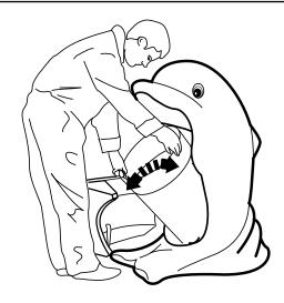
**3.** Tilt forward and lift out liner. After emptying replace liner.
