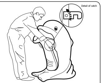
**2.** Whilst lifting both catches, pull door and lift away from Splash.
